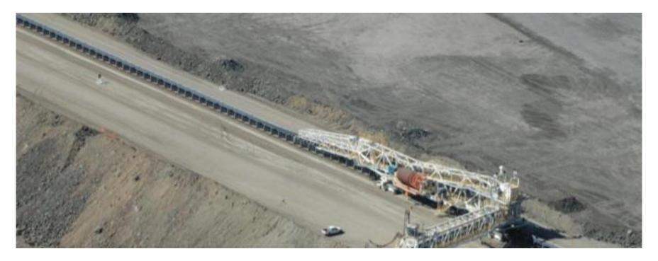
Shifting heads (overland conveyor shifting and aligning mechanisms) attach to the blade arm of a Dozer to relocate the conveyor as required
